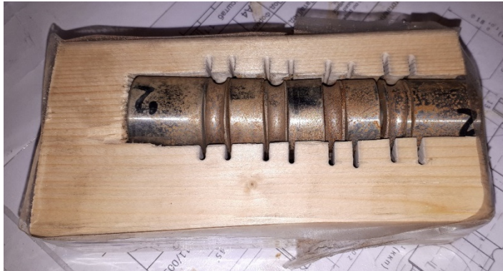
Fig. 9. Transverse shaft cutting into rings
